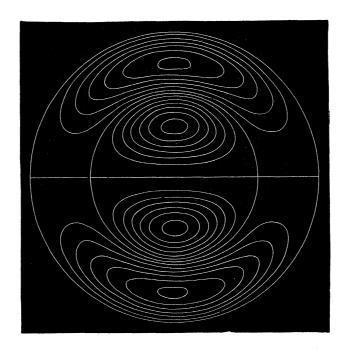
separated by the spheres for which  $\psi_1(kr)=0$ . The drawing includes the first two of these. In the most persistent mode the inner sphere must be taken to represent the boundary of the conductor; in the next mode the second sphere must be taken; and so on.
